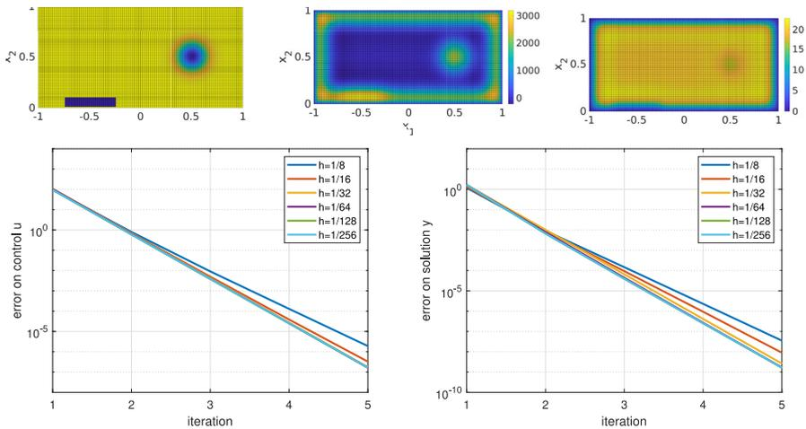
**Fig. 4** Badly insulated room example: heat sinks (top left), best floor heating found by our new DD algorithm (top middle), temperature distribution achieved (top right). Bottom left: convergence of the new DD algorithm for the control  $u$  for different mesh sizes (log scale for the ordinate axis); bottom right: corresponding results for the solution  $y$  (log scale for the ordinate axis)
